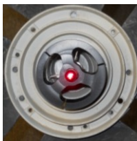
PHOTO A Focal Finder to Locate Center of Antenna
