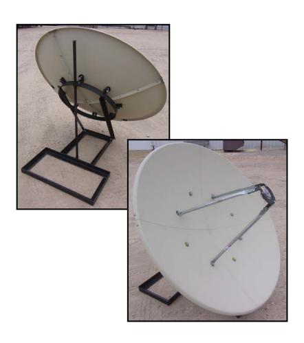
Sectional antennas must be handled with care not to twist or distort sections while handling for installation.
